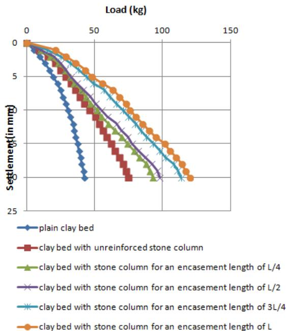
Fig: 6 Load-Settlement curves of clay bed and stone columns having different encasement lengths
