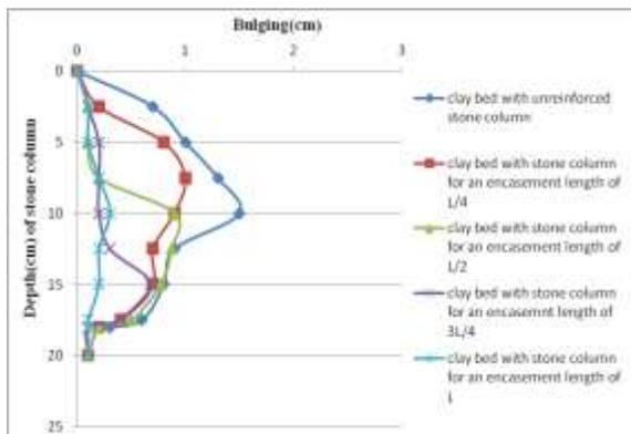
Fig: 7.1 bulging analysis of stone column
