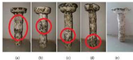
Fig: 7 Deformed shapes of stone columns
