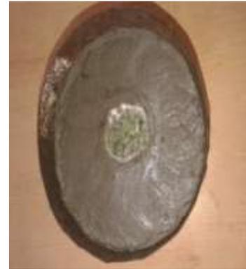
Fig: 4 Stone column with encasement
