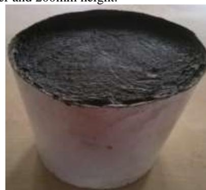
Fig: 2 Preparation of soft clay bed
